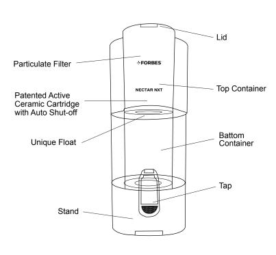
Note: This is a schematic representation/diagram of the actual product to give visual indication of working. This is not an actual engineering drawing of the product.
