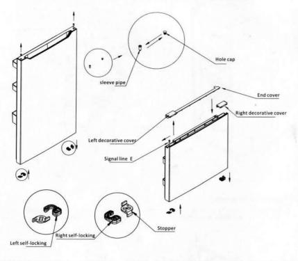
6)Put the refrigerator door on lower hinge vertically, install the middle hinge on left side and two hole caps on right side.
