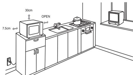
**The rear surface of appliance shall be placed against a wall. A minimum clearance of 3.0 inches (7.5cm) is required between the oven and any adjacent walls. One side must be open.**
