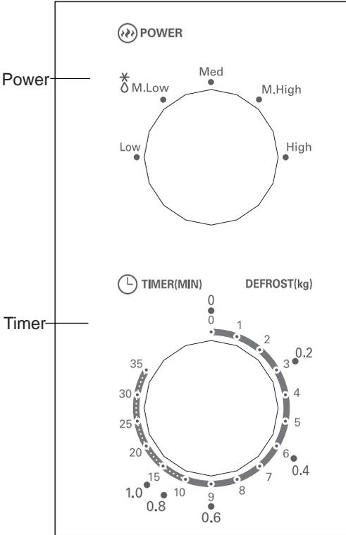
1. To set cooking power by turning the power knob to desired level.
