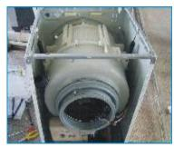
7. Undo the facade counterweight I.Undo the front plate II.Remove six screws pull out the facade counterweight.
