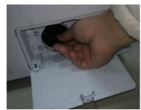
17. Undo the drain pump
