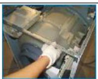
22.Undo the drum tub
