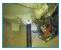
24.Undo the motor I.First let the machine lie down on the back and then pullout the motor wire and grounding wire. II.Use spanner to remove the motor screw, and lift up the motor with the other hand in case of falling to the drain pump III.After two screws are removed, change the motor. First support it to clasp the correct position, then install the screws.
